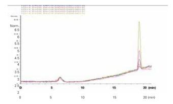
**Figure 1.** High-performance liquid chromatography (HPLC) chromatogram of bisphenol A (BPA) standards. Calculations were made according to the peak heights. Retention times were between 18.3-19.2 minutes
